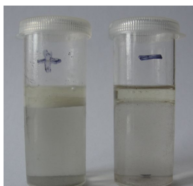
Figure 5. Suspensions formed by intensive mixing of oils with positively charged water do not stratify for hours and, accordingly, retain their milky white or yellowish color (left),
