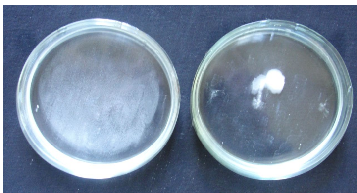
Figure 1. Left: starch powder deposited on the surface of water with a potential of +250 mV. Right: starch powder deposited on the surface of water with a potential of -200 mV [1, 2].
