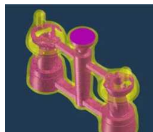
Figure 2 – Determination of shrinkage and porosity when pouring metal molds
