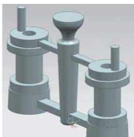
Figure 1 – 3D model of the gating-feeding system
